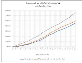
The higher the degree of soiling in the system, the greater the pressure loss. The diagram is based on a clean, new filter insert.
