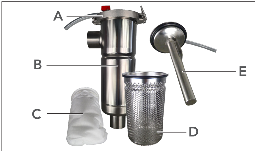
Fig. 3-7: The dual filter in dismantled condition
