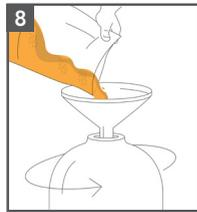
8. Open the refill pack with mixed bed resin and fill it into the composite container using a funnel. If necessary, compact the mixed bed resin by shaking or circling the composite container.
